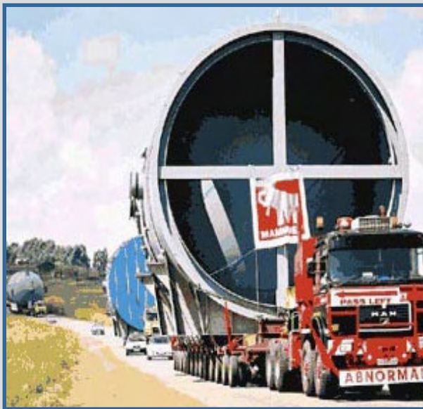
Transporting a FT Pressure Vessel
